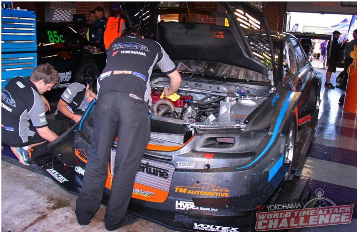
Here we can see the aero package Voltex has created. The front bumper features 2 sets of very large canards, which can be removed to balance the aerodynamic balance (Tilton actually did this in an effort to reduce downforce and maximize speed down the straights). Notice the shallow angle of the canards. The common misconception is that the canard's main purpose is to create downforce. They do create downforce, but their purpose is
