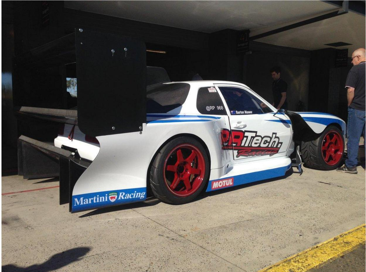
At the rear of the car, we can see are that they diffuser and spoiler now have added gurney flaps. Gurney flaps introduce an immediate obstruction to the air, slowing down the air. This increases the pressure on the high pressure side, which creates a larger pressure gradient when compared to the low pressure side, and aids in keeping the airflow attached. This is why you commonly see them on diffusers and on wings. Speaking of wings, the wing has been moved a bit higher. In our opinion, it
