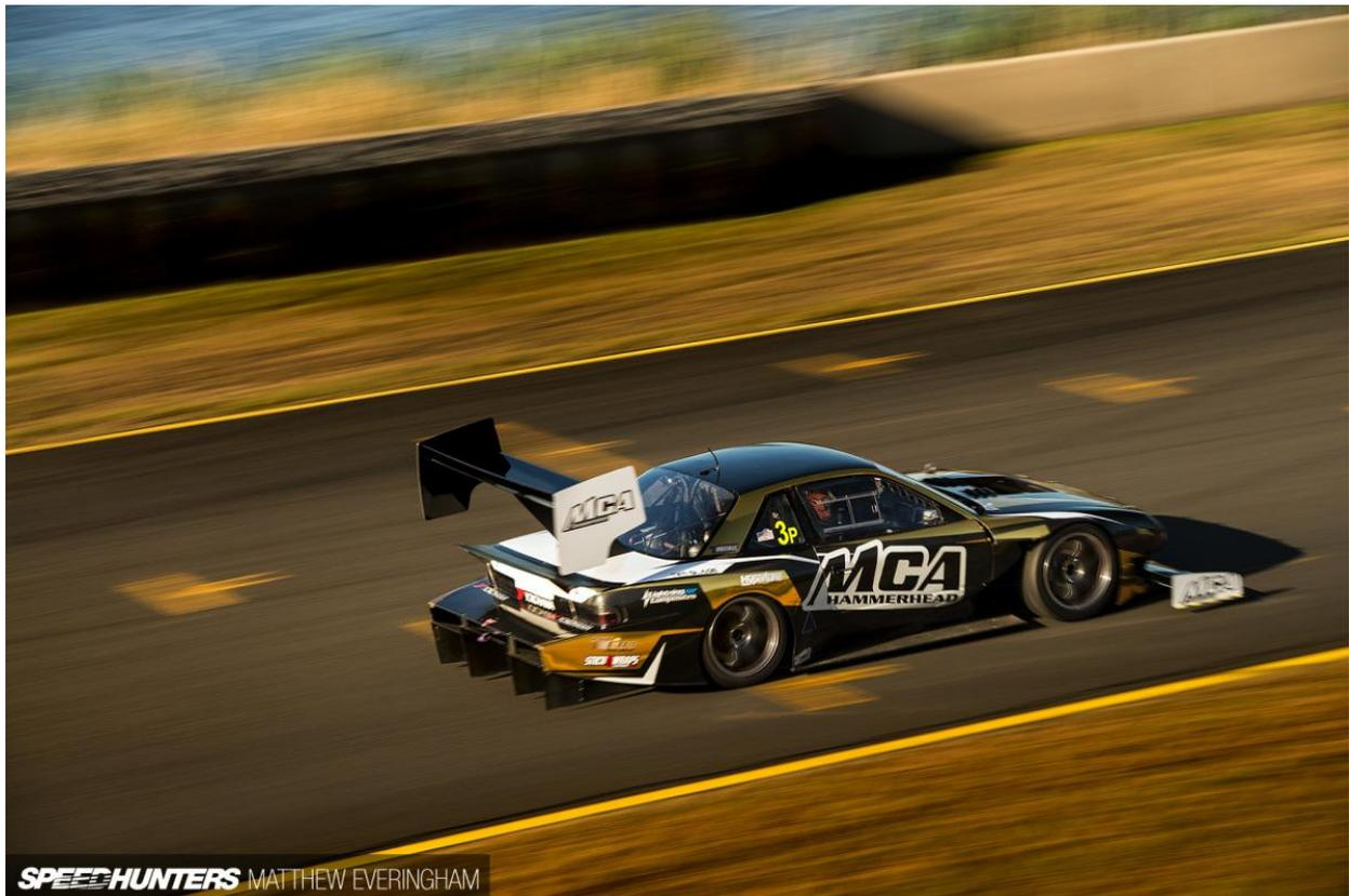
Finally, the rear diffuser of the Hammerhead is a unique design. It has been molded into the “rear bumper” so to speak. Airflow coming off the rear tire and in the rear wheel well is channeled into the upper section of the double diffuser. A double
