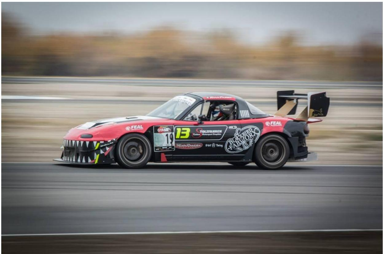
Ryan's car has it all! At the front of the car is a moderate splitter, made of plywood and reinforced with carbon fiber. The splitter features 2 diffuser sections that feed air into the wheel well and out the 2 piece vented fenders. This helps reduce the pressure underneath the front of the car, creating more downforce. Above the splitter is an appropriately sized radiator inlet, which is
